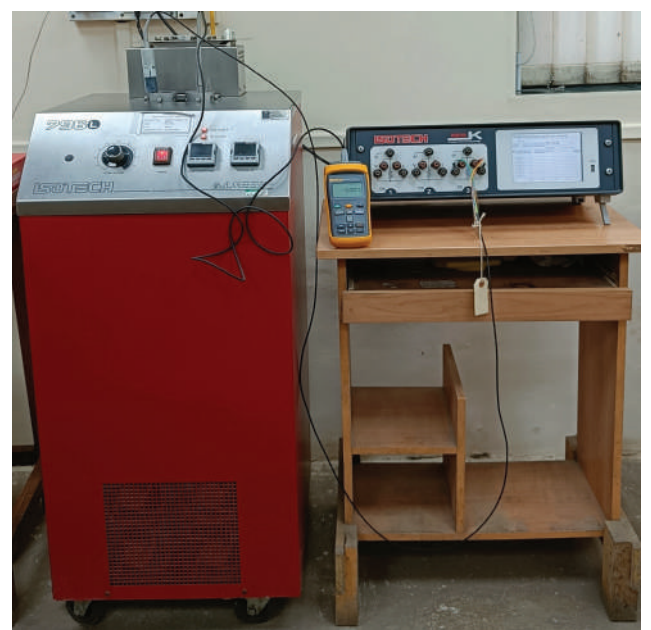
TRIPLE POINT OF WATER(TPW) CALIBRATION USING FIXED POINT METHOD
