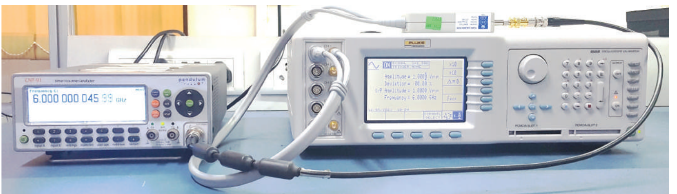
CNT-91 WITH 9500B OSCILLOSCOPE CALIBRATOR
